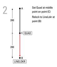
From (C) mid point, go out 200 feet to left and mark your 90° at point (D) using a laser detector 200 CQUAD 200 LINELOKR
