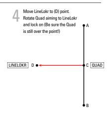
Using a laser detector, go to (A) and (B) and measure where the laser is relative to your (A) and (B) points. This will indicate your square accuracy over the distance from the Quad. (i.e. at 200 feet 1/8 inch= 1/16 per hundred or 10 arc seconds accuracy)
