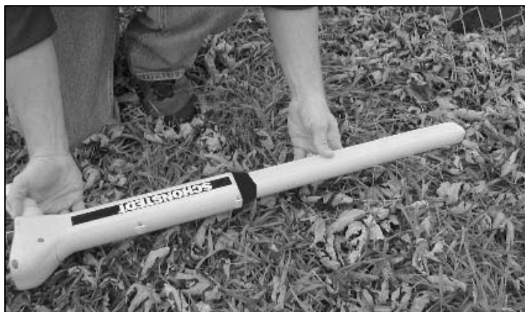
Figure 19. Searching in the Vicinity of a Chain Link Fence
