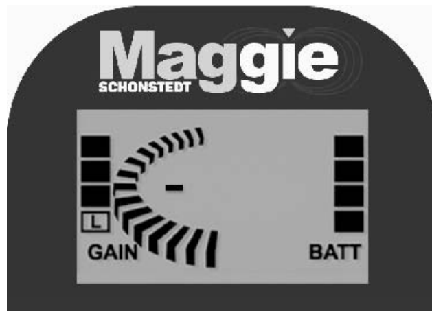
Figure 4. Bar graph and Polarity Indications
