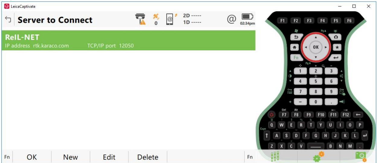
4. Update the Address field to 'rtk.karaco.com' and hit Store. Then hit OK back to the main menu. The address update is complete and there are no other configuration changes needed.
