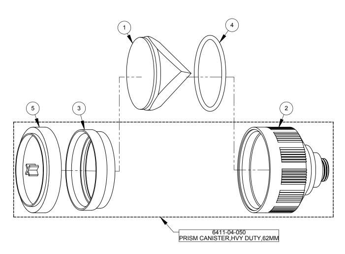
\*NOTE Components may be sold separately. Please see sub-assembly part number drawing for details. ITEM NO. PartNo DESCRIPTION 6411-03-005 PRISM,62MM,SILVER COATED<3' 6411-04-001-BLK HOUSING, PRISM, HVY DUTY, 62MM 6411-04-002-BLK RING,PRISM,HVY DUTY,62MM 6411-04-003 0-RING COVER,PRISM,HVY DUTY,62MM 6411-04-004
