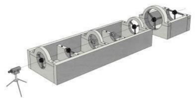
In use, the target is first positioned roughly in the bore center with adjustable feet, then the central target holder is "indicated in". This is achieved using the dial indicator, which is mounted on a sweep arm connected to a rotating central hub. The hub, in turn, contains the optical target. The central hub is adjustable so that it - and therefore the target - may be brought to dead center. This process also reveals and quantifies any out-of-round conditions in the bore.
