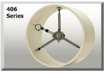
connections (rather than telescoping legs) and the use of "sleds" as feet - no more targets slipping or falling out of bores during your alignment. This feature makes the 406 Series ideal for half-bore and vertical applications. Leg design helps to minimize sag.
