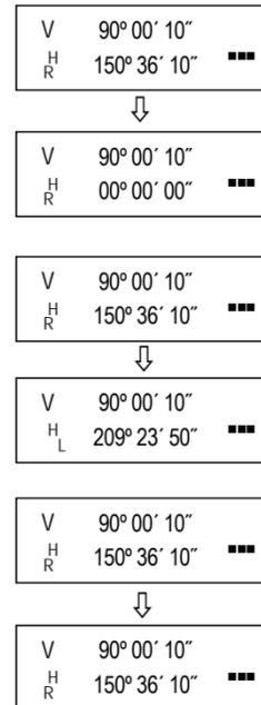
**Selecting the Direction of Measurement of Horizontal Angle.**
