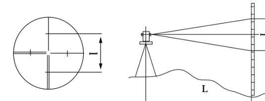
**Perpendicularity of Vertical Crosshair of Reticule of Telescope**
