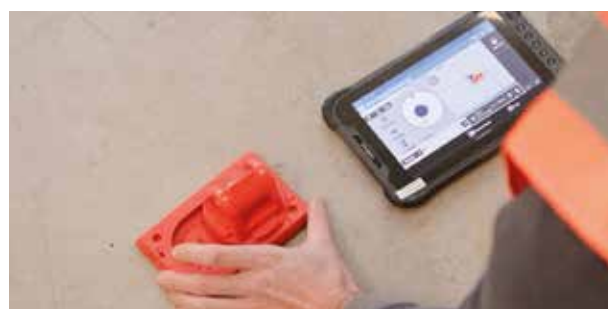
Move the stake out aid on the base plate until the target position is reached – visible on the green circle.
